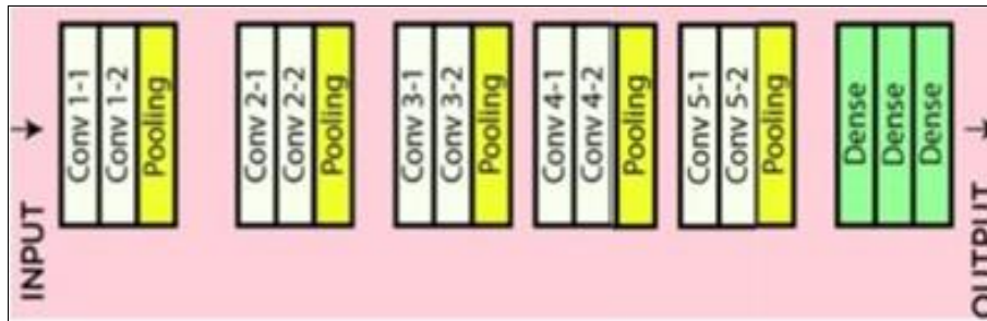
Fig 3: Modified VGG16 architecture
